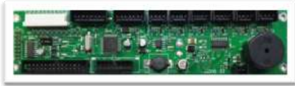
I/O Board Top View
