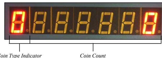
Initially, the machine will be in Continuous Counting Mode, as indicated by a coin count of zero, and the Coin Type will be set to zero (1<sup>st</sup> of 10).
