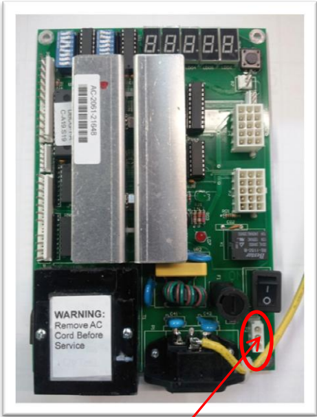
The power supply will connect here.
