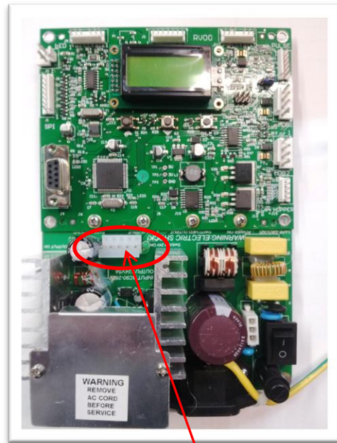
Harness will be connected here.
