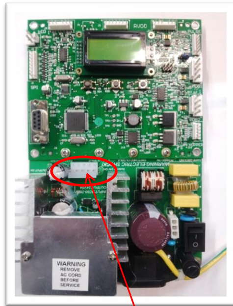
Harness will be connected here.
